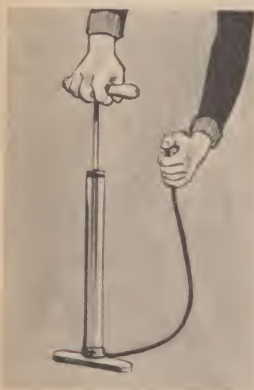
You can easily prove that air is elastic — springy — by compressing it within a bicycle-tire-pump.
